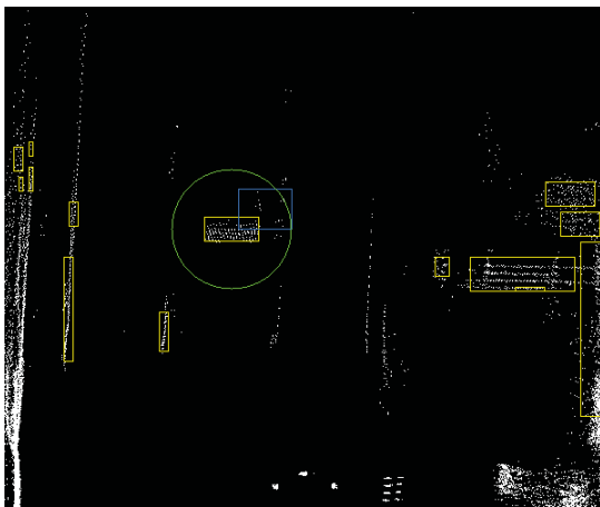
Fig. 11. LIDAR-RADAR object association
